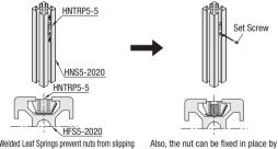
Welded Leaf Springs prevent nuts from slipping off even if inserted into the vertically-oriented extrusions, leading to easy locating
