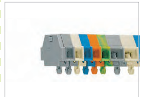
Terminal strip with snap-in mounting feet, for plate thickness 0.6 mm ... 1.2 mm, fixing hole 3.5 mm Ø (fits 210-154 aluminum rail or with 209-120 mounting adapter for DIN 35 rail)
