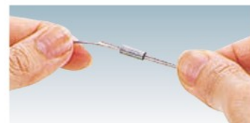
Please stop the wire with the included conforming sleeve.
