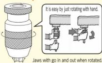
Chuck handle is unnecessary and it is possible to attach/detach the drill by just turning by hand. (automatic tightening mechanism)
