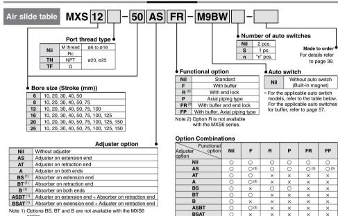
Note 3) When the buffer mechanism and the stroke adjuster on extension end are combined, the buffer stroke will be shorter by the length adjusted by the stroke adjuster on the extension end.
