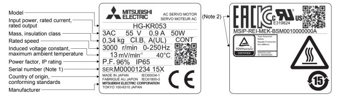
Note 1. Production year and month of the servo motor are indicated in a serial number on the rating plate.
