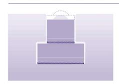
The T-groove type can be used by inserting into existing T-groove without the need for square groove processing.
