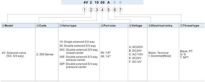
[Note] The wire length is 0.5m. Please refer to P88 for manifold specification and the order way.
