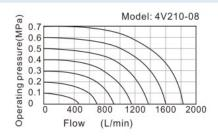
The data in flow rate chart are obtained from AirTAC lab.
